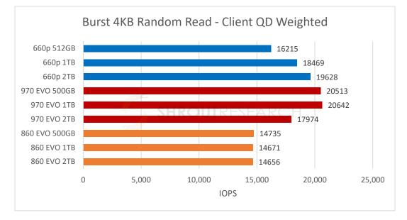
The S-PASS random workload test weighs results based on the Queue Depths commonly observed in client system usage (shown earlier in this paper). In these results, we find the Intel<sup>®</sup> SSD 660p to offer competitive performance which steadily climbs through the higher capacity tiers.
