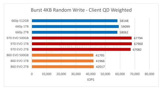
While random writes are less frequently seen on client systems, it is vital that any SSD service them quickly when they do occur. The use of a large SLC cache enables the Inel<sup>®</sup> SSD 660p to remain well within the NVMe performance class, exceeding SATA performance by a comfortable margin.
