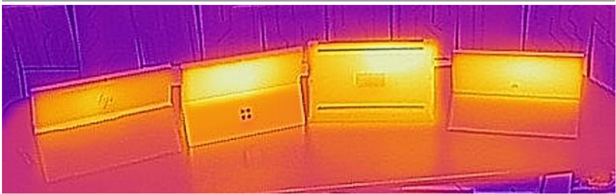
From left to right: HP Envy x2, Microsoft Surface Pro 4, Dell XPS 13 2-in-1, Huawei MateBook E Note: the Dell XPS 13 2-in-1 was placed in a "tent" mode to show the hotspot on the bottom of the machine.
