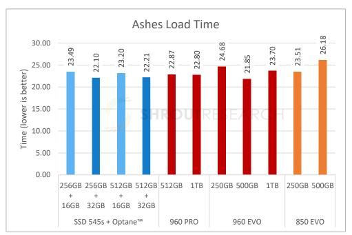
In this graph, we are measuring wall time, so lower is better. The Intel<sup>®</sup> Optane<sup>™</sup> Memory and Intel<sup>®</sup> SSD 545s combinations are consistently on-par or faster than the best NVMe SSD options on the market including the 960 PRO and 960 EVO.
